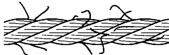
Broken Strand Wires
