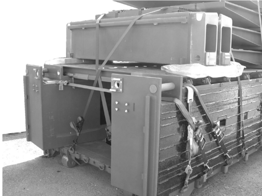
Figure 11. 104 T1- Ramp, Approach Ramps, Access Ladders and End Beams Diagonal Strapping
