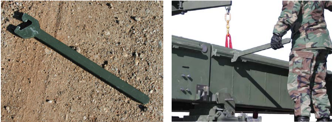
Figure 3.42 End Beam Wrench and Method of Use
