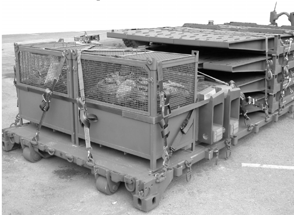
Figure 11. 111 T3 Flatrack End Strapping
