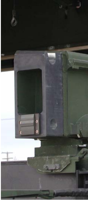
Ramp Module End Beam
