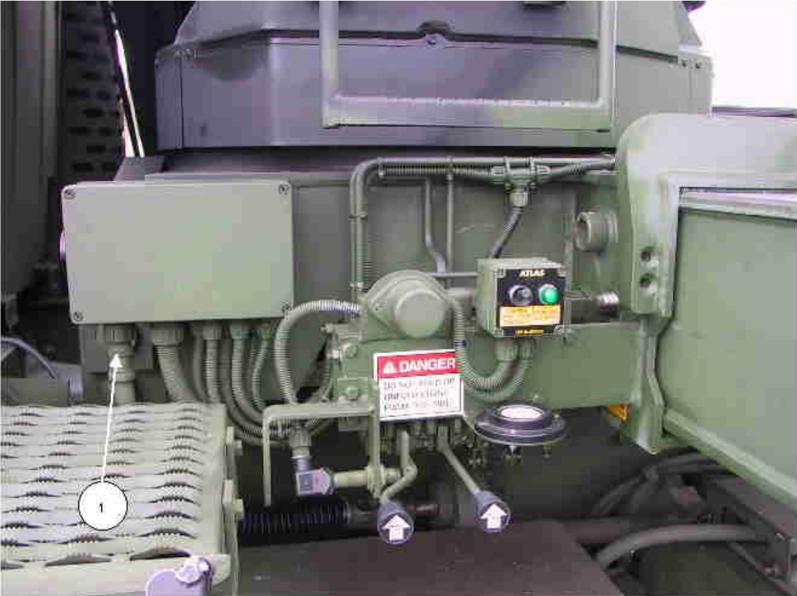
Figure 11. 56 Crane Electrical Connection
