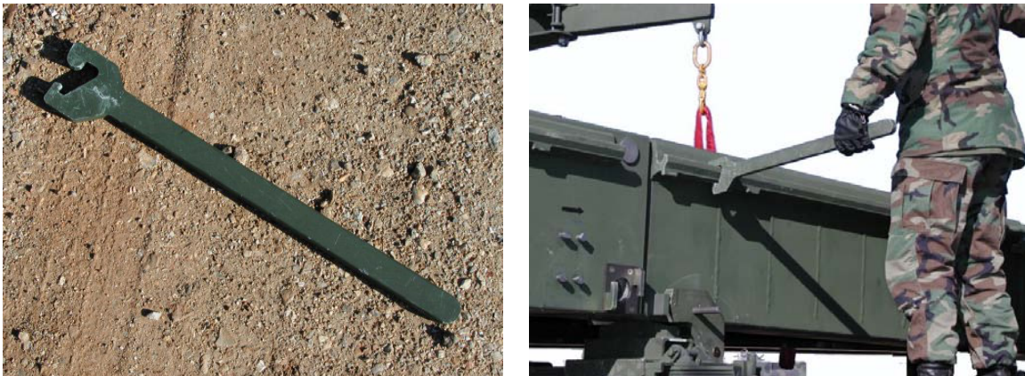
Figure 4.13 End Beam Wrench and Operation
