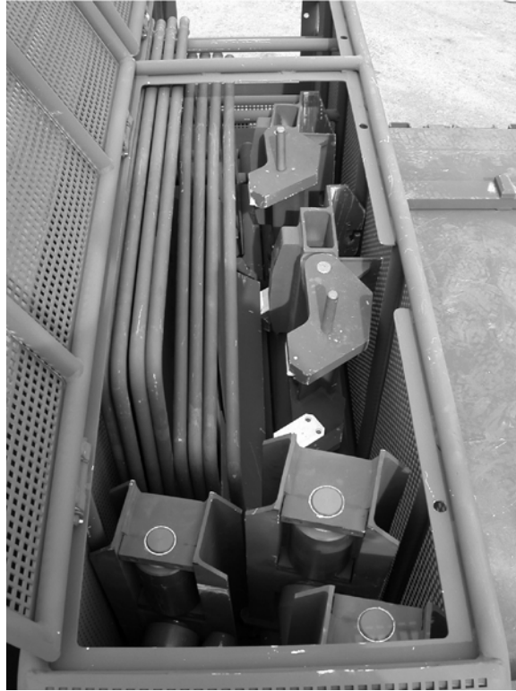
Figure 11. 123 Ramp End Beam Adapter Stowed
