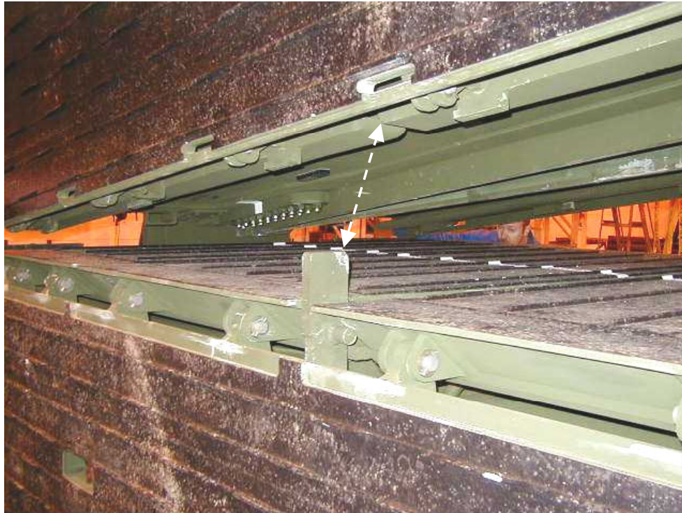
Figure 3. 54 Lower Top Module Onto Aid
