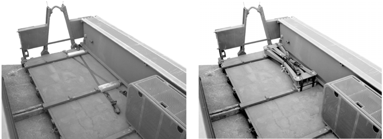
Figure 11. 118 Bridge Module Lifter Folded and in Position on LVT Flatrack
