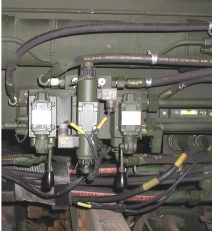
Figure 3. 25 A-Frame Stabilizer Controls
