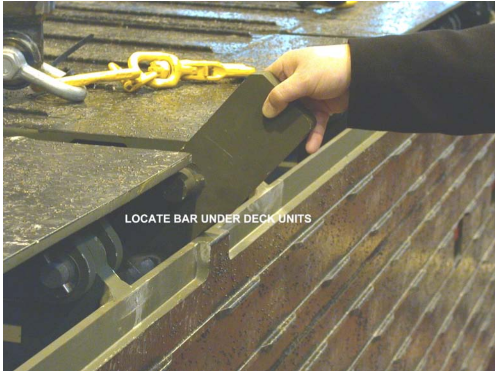
Figure 11. 100 Transport Aid Inserted Under Deck Unit
