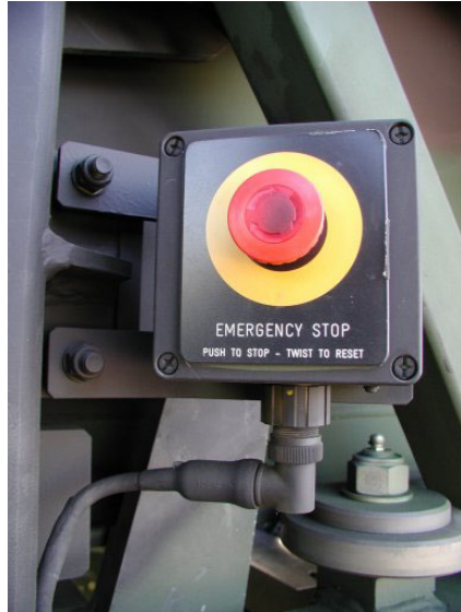
Figure 2. 22 Example Emergency Stop
