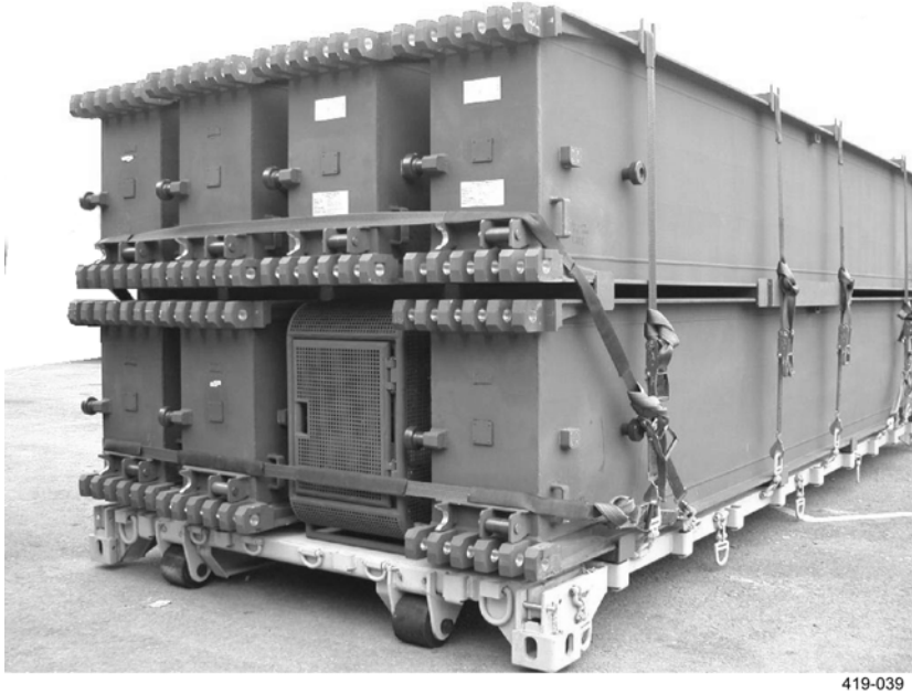
Figure 11. 113 Flatrack LVT Load Strapping
