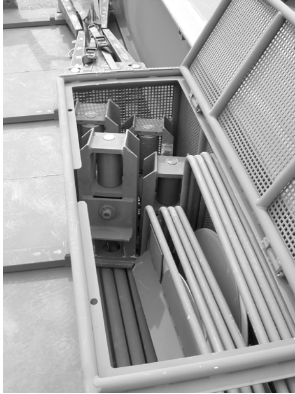
Figure 11. 121 Tail-lift Handrails and Removable Rollers Stowed
