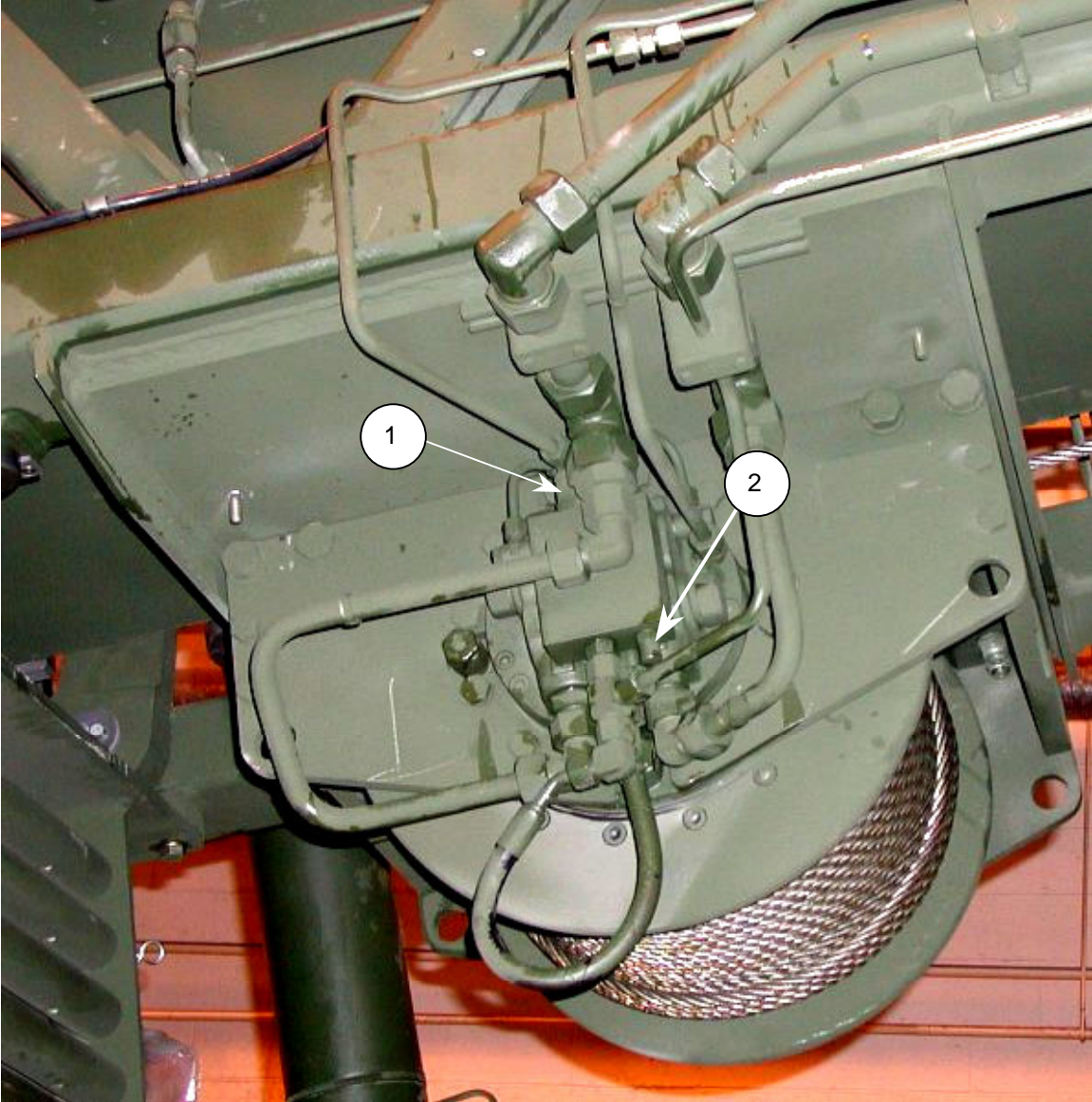
Figure 10. 38 Lower Winch Pilot Valve Adjustment
