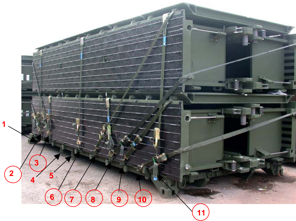
Figure 11. 96 T2 - Parallel and Parallel Module (End Strapping)
