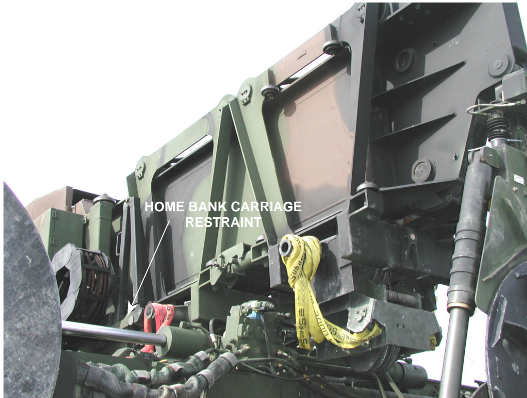
Figure 3. 37 Home Bank Carriage to Launch Frame Restraint
